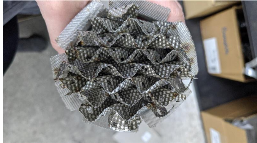
Commercial packing (Mellapak 250)
