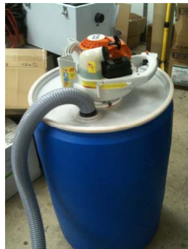
Fig. 5. FOG siphoning unit. Drum can be mounted on a tricycle. An operator could service 50 to 100 restaurants.
