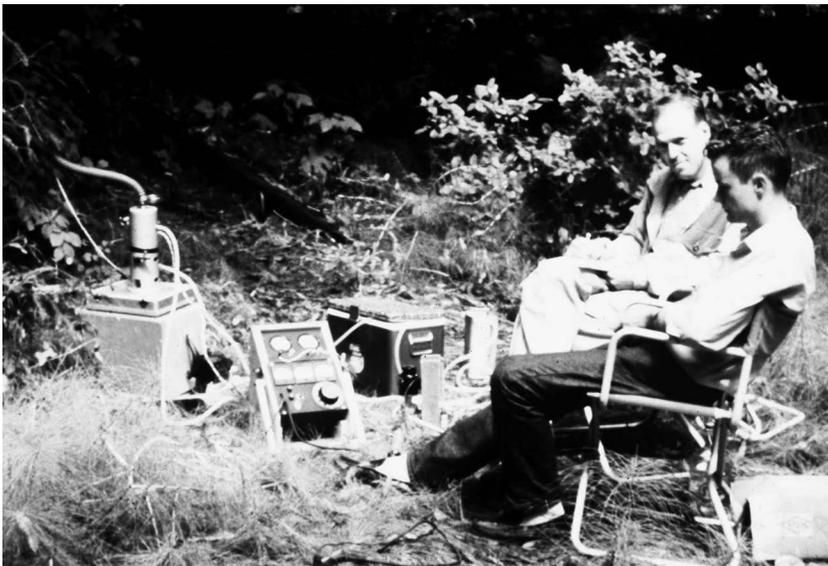
*Figure 2. Othmar Preining (left) measuring with the Goetz aerosol spectrometer (far left) in Sequoia National Park, 1958.*
