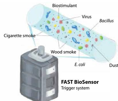
The FAST BioSensor provides a means for total aerosol concentration and bioaerosol detection in real time.
