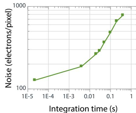
(Left) Plot of the FPA spectral QE. QE shown is the mean response for the array under monochromatic illumination. The FPA exhibited an average QE of 15% across the spectral range shown. (Right) Total per pixel RMS noise electrons as a function of integration time plotted on a log-log scale.
