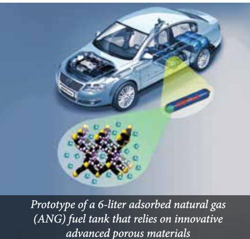
Prototype of a 6-liter adsorbed natural gas (ANG) fuel tank that relies on innovative advanced porous materials
