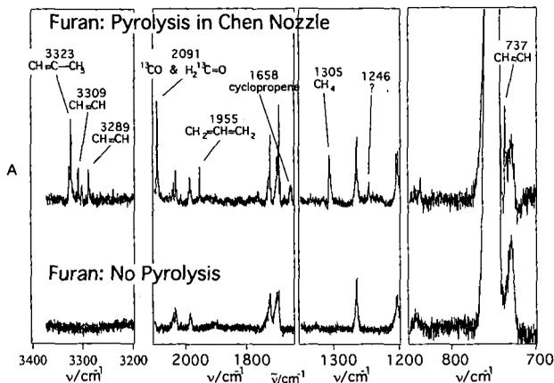
**Figure 7** Matrix isolation FTIR spectrum of the pyrolysis products of furan (top) compared to the spectrum of furan alone.
