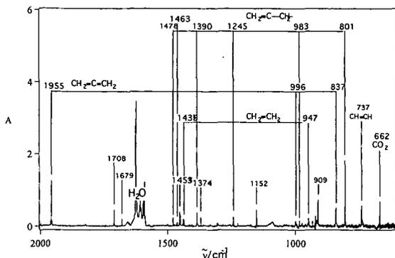
**Figure 5** Matrix isolation FTIR spectrum of the products obtained from the pyrolysis of allyl iodide in a Chen Nozzle. Allyl radical ( $\text{CH}_2=\text{CH}-\text{CH}_2^\bullet$ ), allene ( $\text{CH}_2=\text{C}=\text{CH}_2$ ), ethylene ( $\text{CH}_2=\text{CH}_2$ ), and acetylene ( $\text{CH}\equiv\text{CH}$ ) are identified in the spectrum
