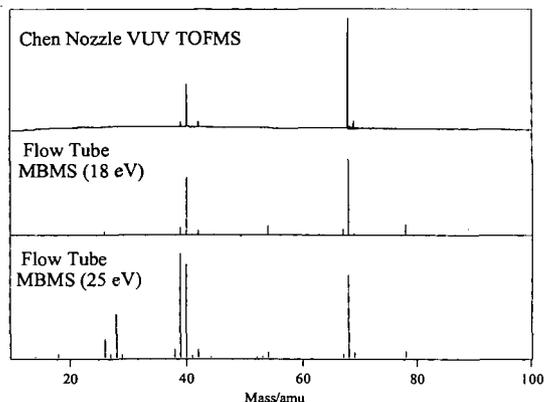
**Figure 2** Mass spectra of the pyrolysis products of furan. The top spectrum shows the products from pyrolysis in a Chen Nozzle while the bottom two spectra show products from a heated flow tube reactor (1 cm i.d., ~1 sec. residence time, 750 °C).
