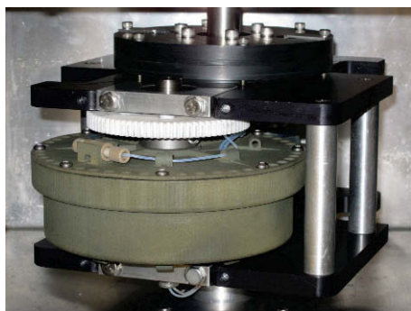
Fig. 1. The STS rotor made of nylon polymer plastic mounted in a planetary centrifuge [3].
