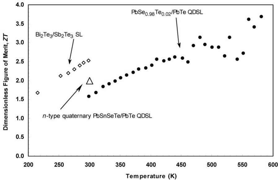
Figure 1. Thermoelectric figure of merit  $ZT$  for  $\text{Bi}_2\text{Te}_3/\text{Sb}_2\text{Te}_3$  superlattices<sup>3</sup> (SL),  $\text{PbSnSeTe}/\text{PbTe}$  quantum dot superlattices (QDSL), and  $\text{PbTeSe}/\text{PbTe}$  quantum dot superlattices.<sup>4,45</sup>
