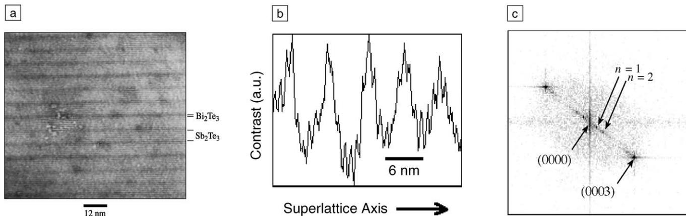
Figure 3. (a) Transmission electron micrograph of a  $\text{Bi}_2\text{Te}_3/\text{Sb}_2\text{Te}_3$  (10 Å/50 Å) superlattice. (b) Image contrast oscillations through the superlattice. (c) Fast Fourier transform of the image in (a), showing the superlattice reflections of order  $n$ .<sup>22</sup>
