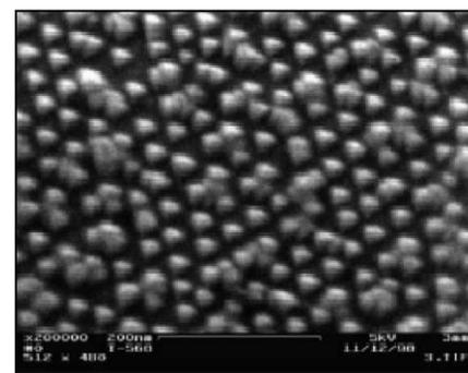
Figure 4. Quantum dot structures in the  $\text{PbTe}/\text{PbSeTe}$  system.<sup>42</sup>
