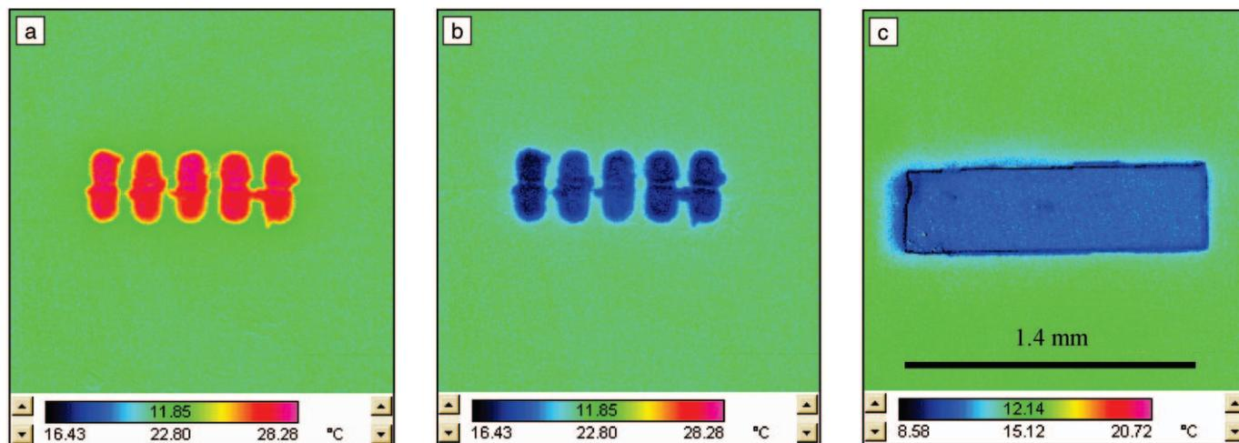
Figure 5. Infrared image of a row of five  $\text{Bi}_2\text{Te}_3$ -based thermoelectric superlattice microcoolers. (a) Discrete heating; (b) discrete cooling. (c) Combined discrete cooling devices for larger-area cooling. The scale marker in (c) applies to all three images.
