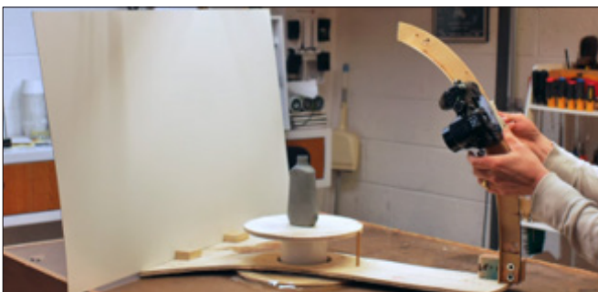
Figure 2: The turntable method, as shown on the left, provides more consistency in photos, and is a quick method to capture smaller objects.
