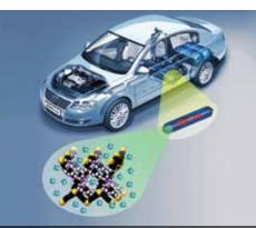
Prototype of a 6-liter adsorbed natural gas (ANG) fuel tank that relies on innovative advanced porous materials
