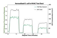
A preparation of *E. coli* bacteria was aerosolized and injected into a ventilation test duct at three different times and concentrations. In this test, because the bioaerosol used was mostly bacteria, the APS concentration should mirror the bioaerosol detection by the FAST.
