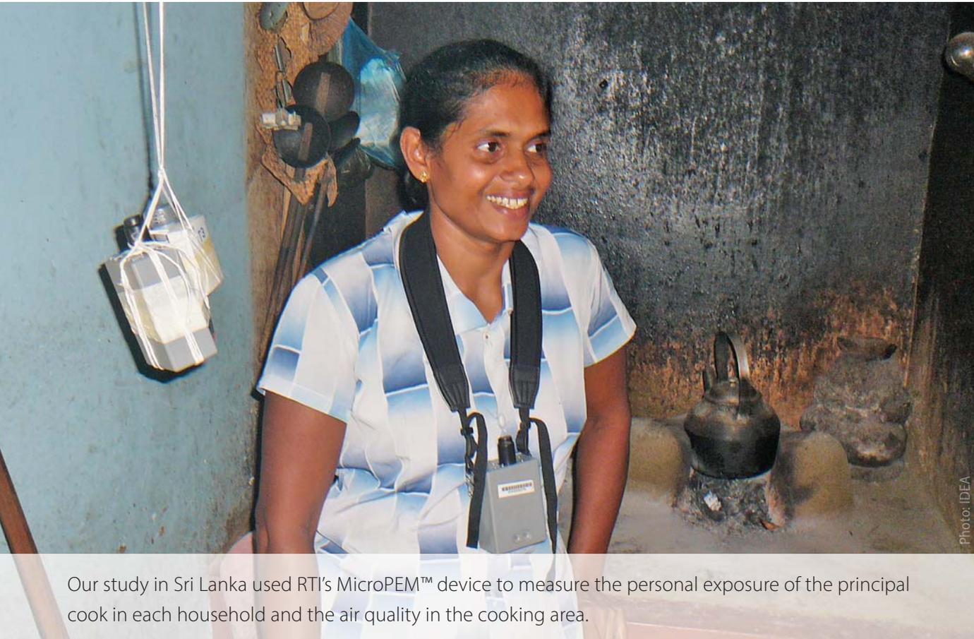
Our study in Sri Lanka used RTI's MicroPEM™ device to measure the personal exposure of the principal cook in each household and the air quality in the cooking area.
