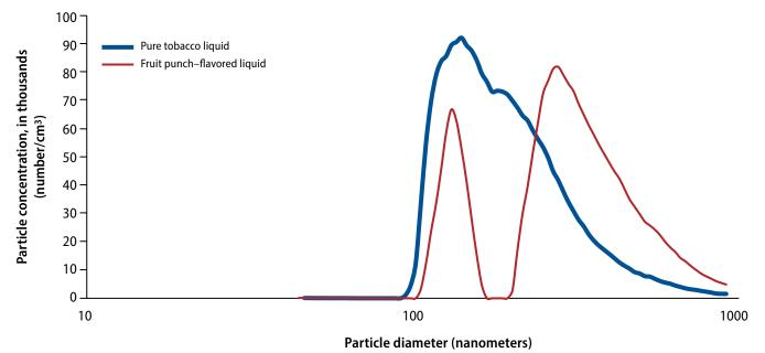
Note: The e-cigarette was connected to a temperature- and humidity-controlled chamber to simulate a user's respiratory system.
