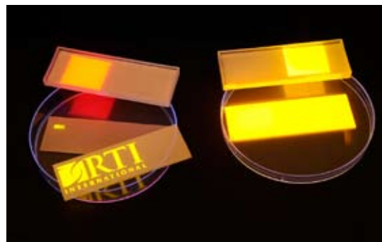
Figure 9. A variety of patterns ranging in size from very small to coverage of the entire substrate are being produced with the current RTI technology of spray coating QDs onto nanofiber mats.
