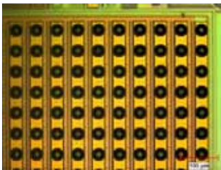
25 micron diameter bumps on 50 micron pitch
