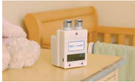
RTI's MicroPEM™ for assessing particulate matter exposure
