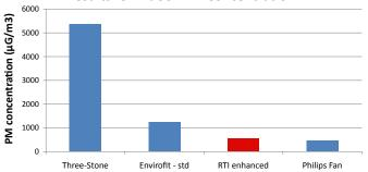
With the RTI insert, emissions from a commercial cookstove were significantly lower than emissions from the traditional three-stone fire.
