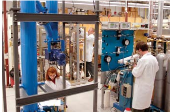
RTI's bench-scale Dry Carbonate CO 2 Removal Process
